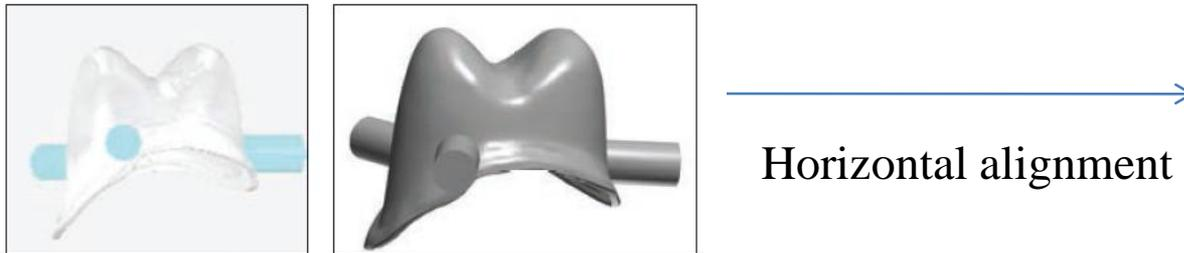
■ When milling multi-unit restorations, the bars should be attached on the oral and the vestibular side of the restoration.
