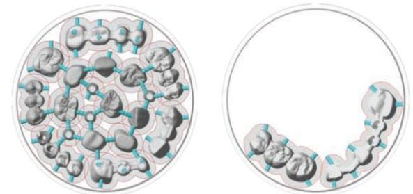
The distance to the edge of the disc is monitored by the disc edge control function of CAM. This means that it is not possible for the object to extend beyond the edge of the disc. If the disc edge control function is deactivated, it is important to ensure that the object does not extend beyond the edge of the disc. Extension beyond the edge will be highlighted in red.
