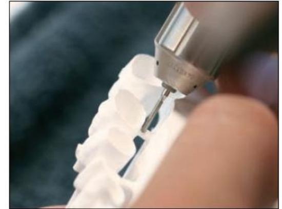
*6. Separate bars attached to the sintering tongue which are not required.*
